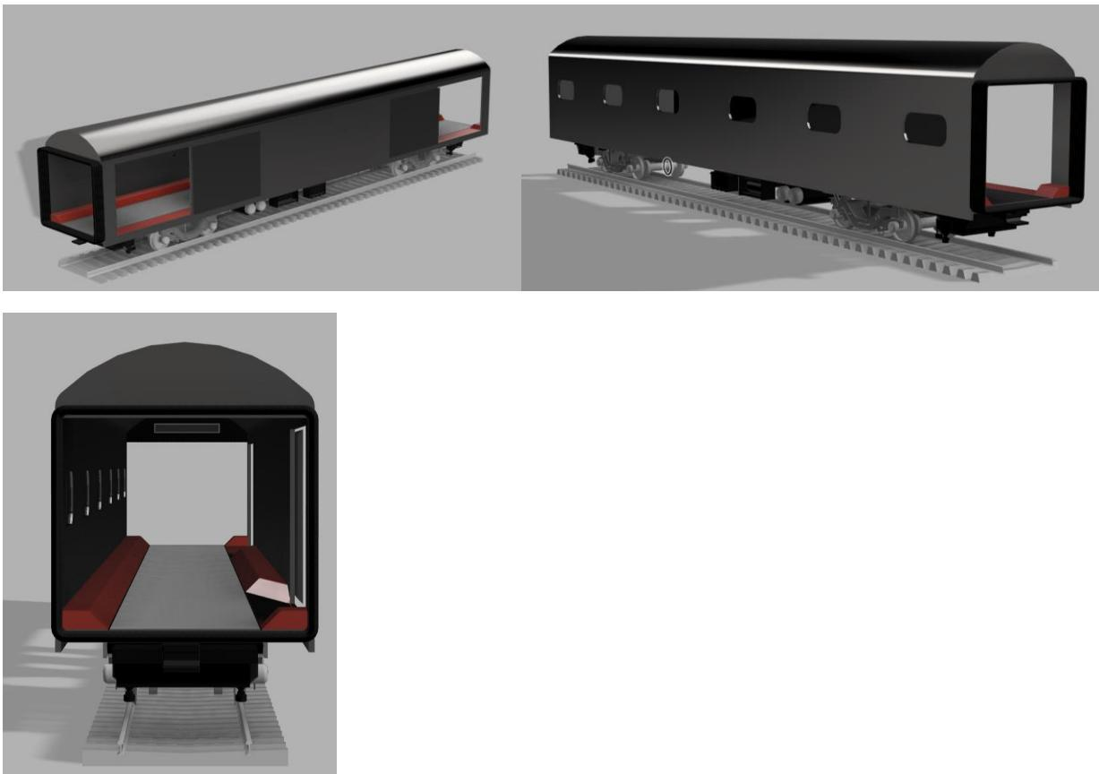
The train ferry car's interior is structured with side ramps curbs for guiding elements to secure vehicles during transit, providing stability and preventing lateral movement. The car's interior dimensions are adaptable, allowing it to accommodate a range of vehicle sizes, from standard sedans to larger SUVs and trucks. Reinforced side walls and a robust flooring system enhance durability, while strategically placed windows allow for visibility.
